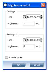
Set the desired times and the corresponding brightness levels. Activate the timer and confirm your settings with OK.
