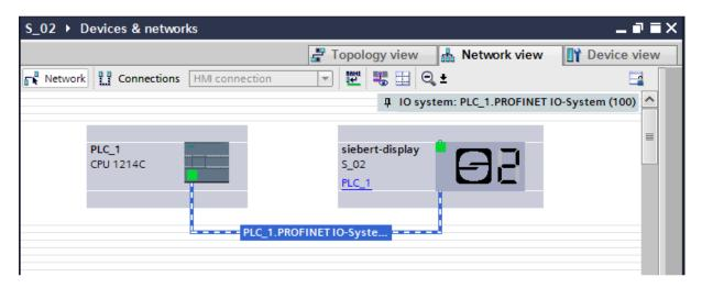
Assign the display to the desired control in the network view. Then the PROFINET connection is shown.
