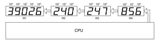
Data telegrams sent to the display are valid for either a specific display field or for all display fields (see chapter 'Data format').
