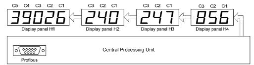
The control computer takes over the conversion from binary format to decimal format in all display fields.
