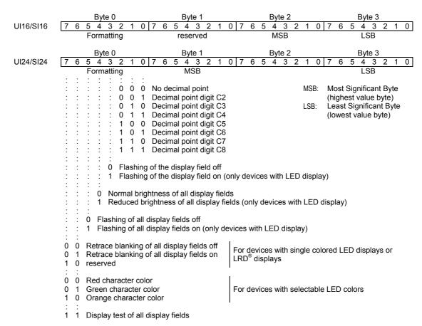
The formatting for the brightness, flashing of all display fields, retrace blanking and display test can be set in byte 0 of the display field H1. The bits in the other display fields should be set to 0 in byte 0.
