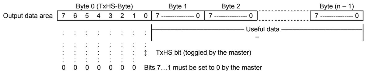
For the busy check, bit 7 (RxHS bit) has been reserved in the only byte of the input data area (RxHS byte). Bits 6...0 are read by the master as 0.
