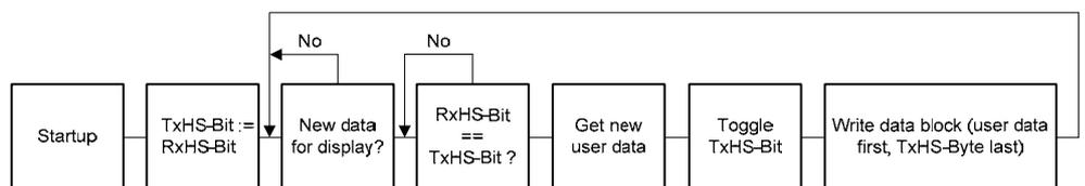
The display is ready to receive as soon as the RxHS bit has the same value as the TxHS bit sent last. Now the master can send new data to the display. The master marks new data by inverting the TxHS bit (toggle). After a short time, the display signals again readiness to receive by setting the RxHS bit equal to the TxHS bit received last.
