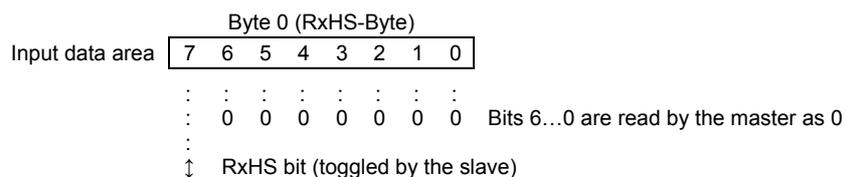
**Flow chart**                                During the start, the master must set the TxHS bit to the value of the RxHS bit.
