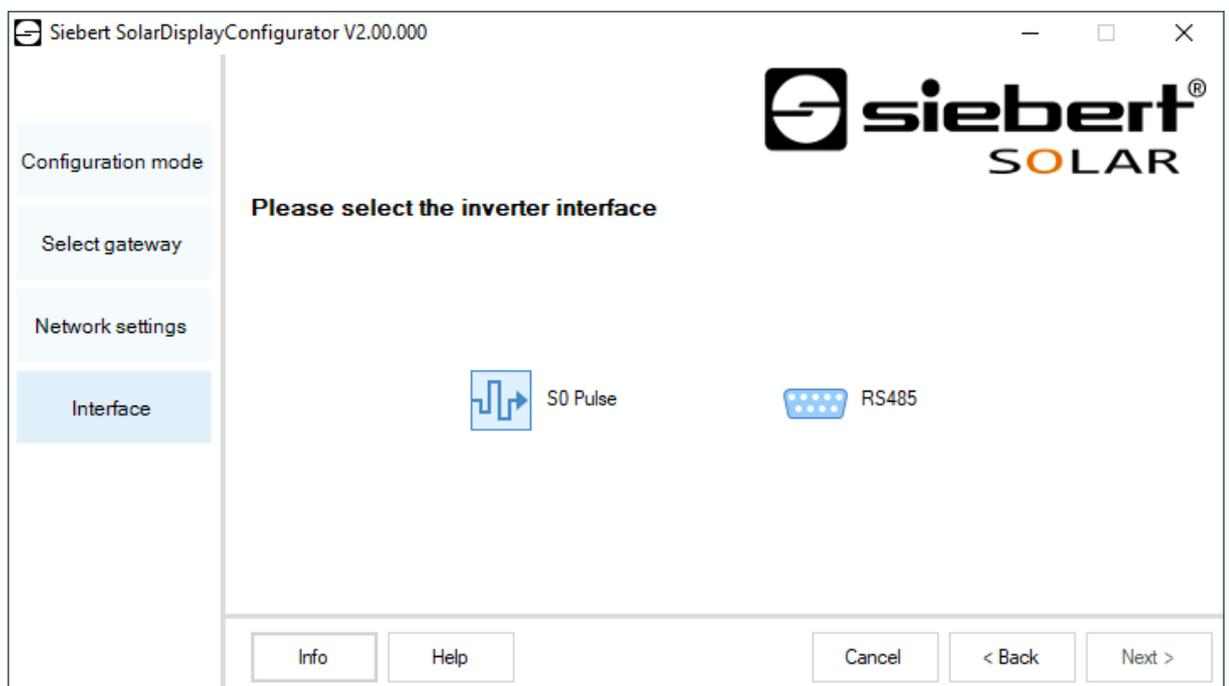
If you are in 'Gateway' mode, you must select the interface of the inverter to be connected to the Siebert Ethernet Gateway. The data of the inverter can then be queried and displayed by a Siebert solar display with an Ethernet interface from the Siebert Ethernet Gateway.
