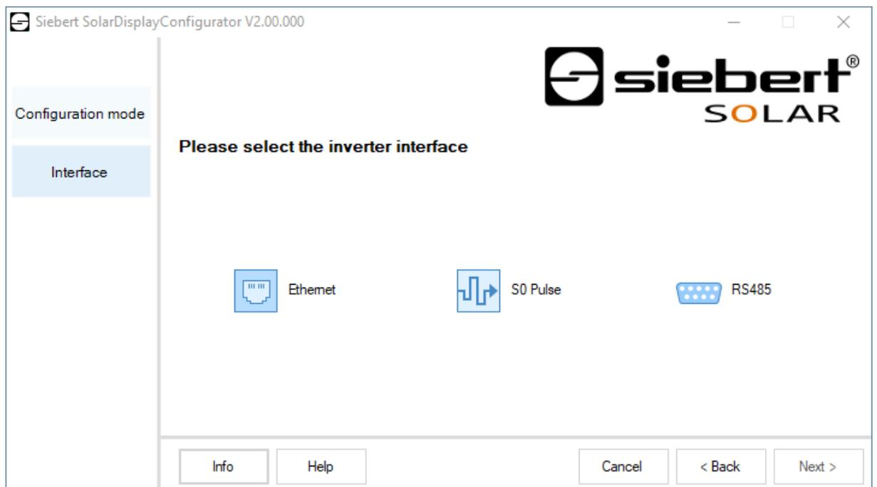
If the inverter, resp. the data logger is connected to the display via a S0 interface, resp. a pulse exit, please select 'S0 Pulse'.
